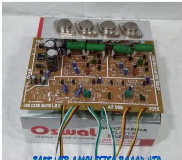
3055 USB AMPLIFIER BOARD 4TR.
