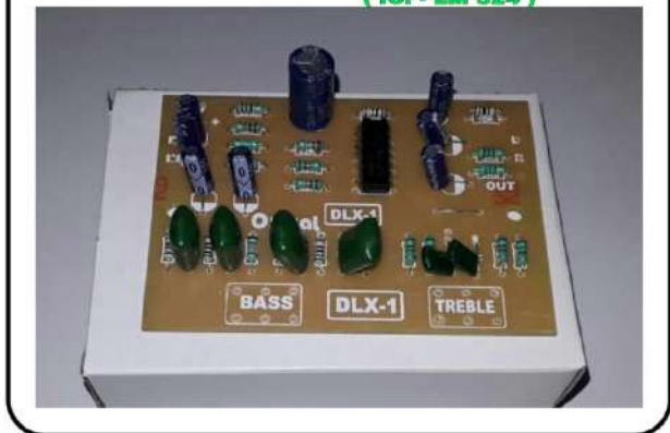
BASS TREBLE BOARD ( IC. - LM 324 )
