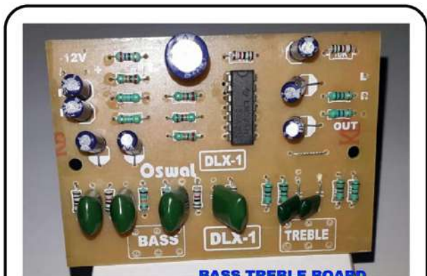
BASS TREBLE BOARD ( IC. - LM 324 )
